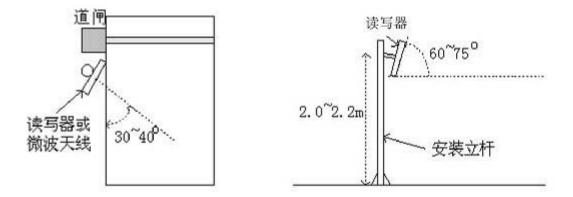
Antenna pitch: refers to the angle between the antenna tilting to the ground and the horizontal line, about 60 to 75degrees
