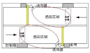
On-site installation mode 2: the road has an intermediate isolation of the safety island, control equipment (gate) installed in the middle of the isolated safety island, vehicle speed of less than 10 km / h through the card reading area.
